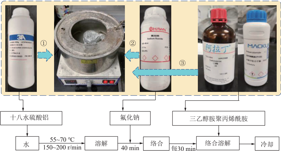
图 7 复合外加剂制备工艺流程 Fig.7 Process flow for the preparation of composite additives
