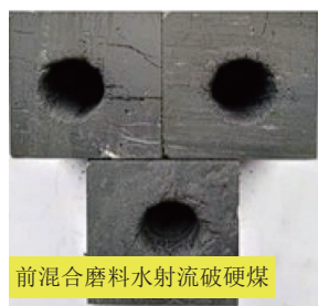
Fig.45 Comparison of rock-breaking effect of pre-mixed abrasive water jet and over-mixed pulsed abrasive water jet
