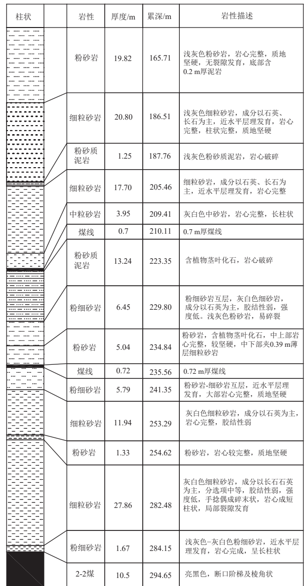
图1 开切眼前方1000 m位置煤层上覆100 m范围内岩层赋存 Fig.1 Occurrence of rock strata in the range of 100 m above the coal seam at 1000 m in front of the open-off cut
