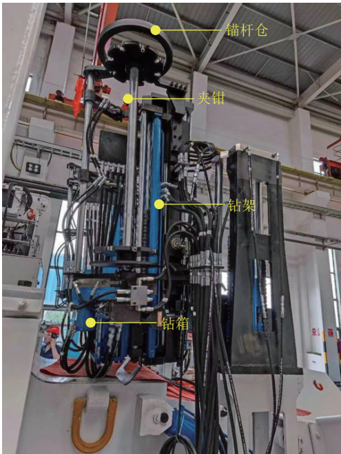
图 7 钻锚一体化锚杆施工装备 Fig.7 Construction equipment of integrated drilling and anchoring bolt
