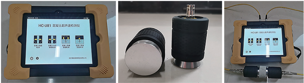
图 3 冲击性岩样超声波检测 Fig.3 Ultrasonic detection of impact rock samples
